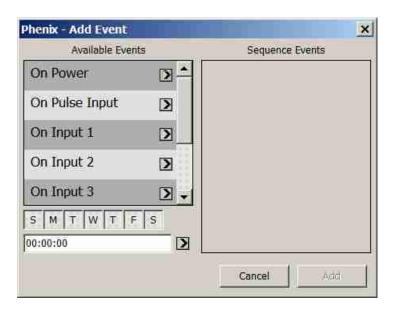
• The Model 9262 can have either events happen on power up or days and times of the week. Also input events are available on the 9262. So select either "On Power" or add days and times of the week or inputs events to trigger the start of a sequence. The arrow to the right of each event will add it to the list of events that will start the sequence.
