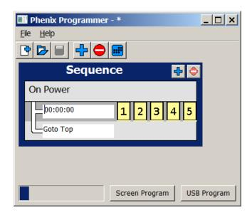
• This is where you add to the sequence and select what output will be on. The blue "+" next to sequence will add steps to the sequence. Edit the text boxes for the time for each step and click numbers that correspond to the output you want to use. Powering on starts this sequence example:
